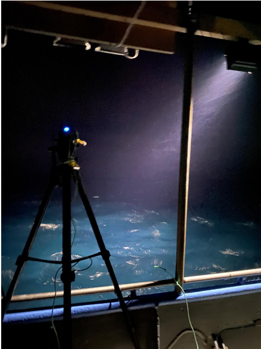
Figure 10. Light array (LED flood illuminated) and thermal scope in action on board the Southern Cross , off the Mercury Islands. Winds gusting 40 kns were not forecast. Photo: Chris Gaskin
