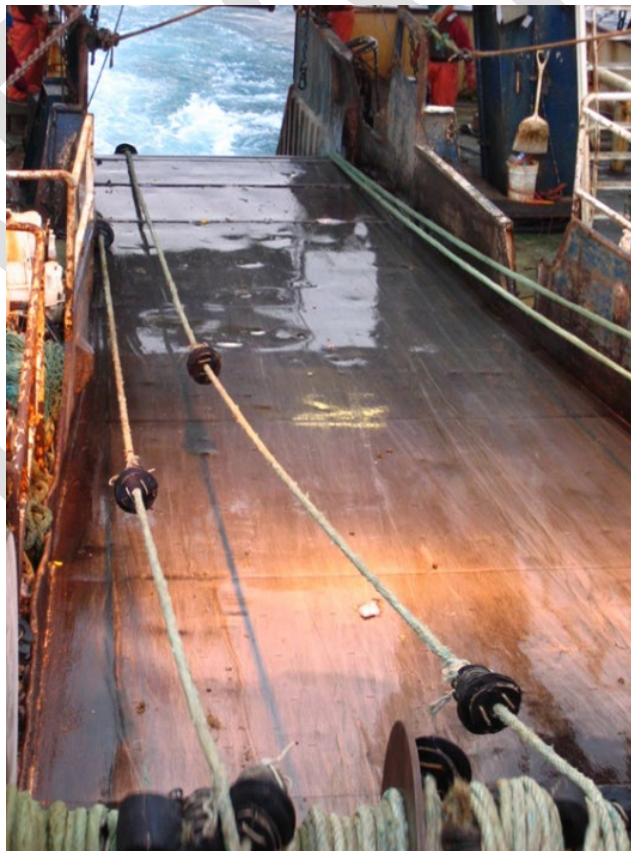
Plate 5. Cluster discs attached to trawl sweeps. Source: J. Gauvin. Alaska Seafood Cooperative.
