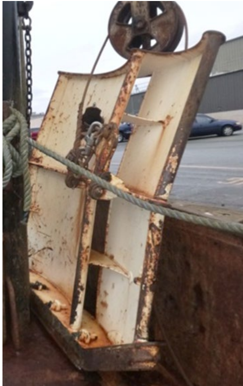
Plate A-4. The Gull wing otter board. Image courtesy of P. He.
