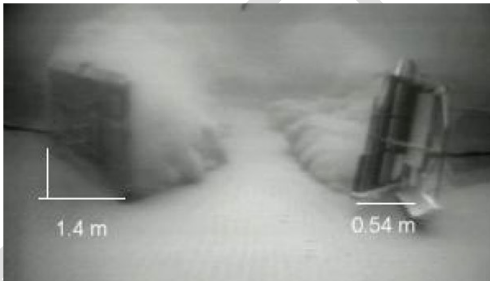
Plate 3. The effect of angle of attack on the swept width (footprint) of otter boards. The flat rectangular otter board on the left is operating at an angle of attack in excess of 30^\circ and the 'batwing' otter board on the left is operating at around 20^\circ . Source. Sterling and Eayrs, 2010.
