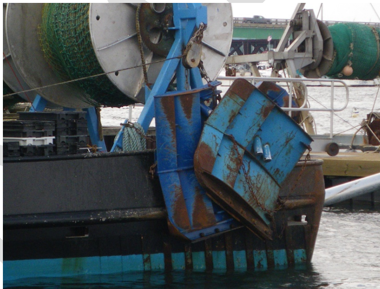
Plate A-3. The traditional otter board (outside) and the semi-pelagic otter board (inside). Note the difference sizes of each otter board. Image courtesy of S. Eayrs.
