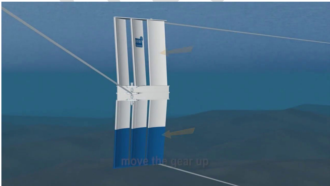
Figure 21. Controllable otter boards. By opening the upper vents and leaving the lower vents closed, otter board height above the seabed is increased. Source: Notus electronics.
