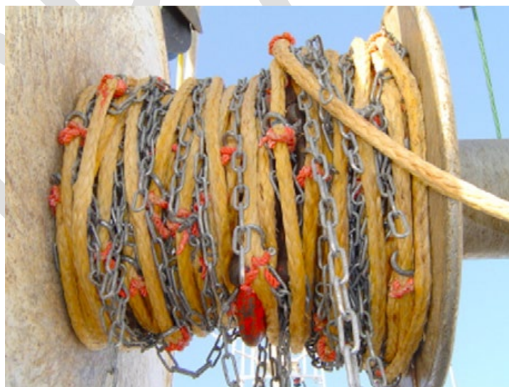
Plate B 3. Chain droppers attached to a dyneema sweep. Source: Guyonnet et al. , 2008.
