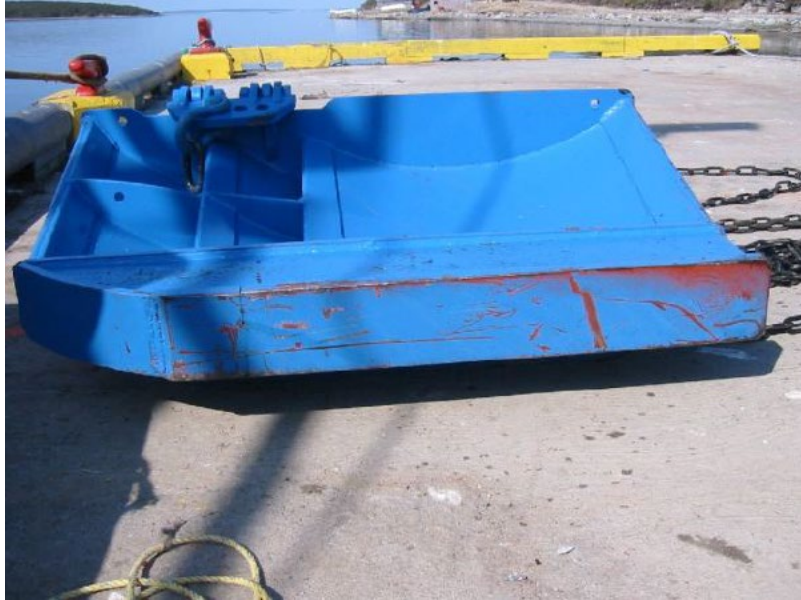
Plate A-1. Shoe of semi-pelagic otter board indicating limited seabed contact.
