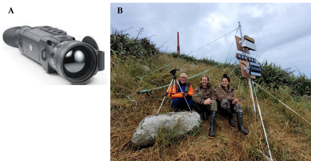
Figure 4. (a) Image of the Pulsar Helion XP38 thermal imaging camera and (b) relative position of tripod to the lighting rig
