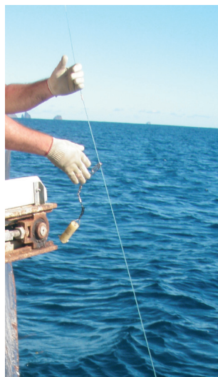
Time-depth recorders (inside the yellow cylinder shown here) were used to measure longline sink rates during the project. Photo: DOC
