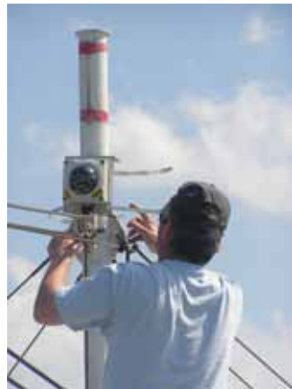
A camera being fitted to an Australian vessel for electronic monitoring. Photo: www.afma.gov.au/category/uncategorized/
