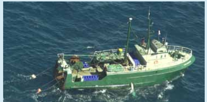
Seabird bycatch reduction devices deployed astern a trawler fishing in Australia's South East Trawl fishery. Photo: http://www.afma.gov.au/2012/07/fishers-lift-game-for-perfect-compliance-with-seabird-rules/ .
