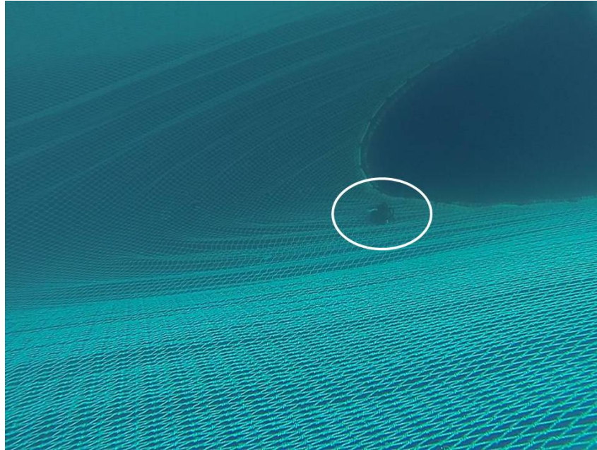
Figure 9: Camera (circled) deployed in the centre net of a triple-rig scampi trawl.
