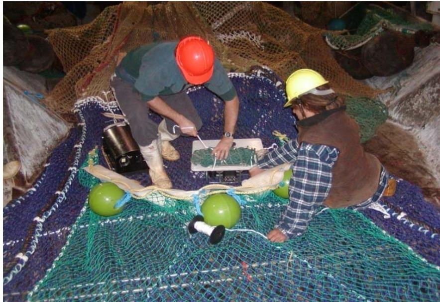
**Figure 1:** Deck crew fitting the cameras to the SED with netting packing to improve field of view, *FV Taimania*, April 2009
