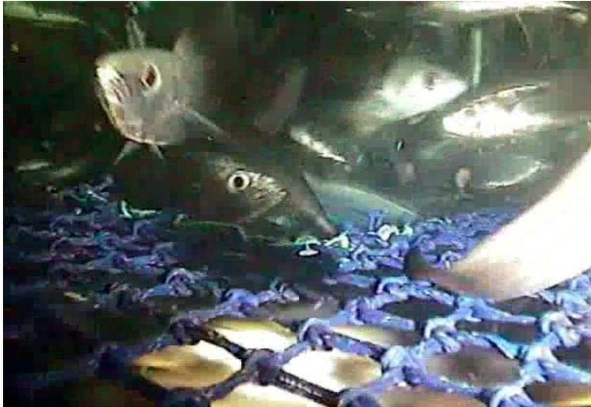
**Figure 9:** Hoki swimming freely from escape hole of SED during high catch rates achieved during initial trials, Cook Strait, 2008
