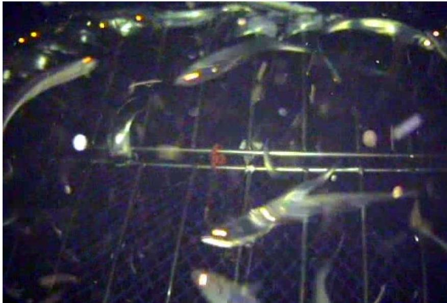
**Figure 15:** Video still of hoki impacting on grid bars during tow. Note sideways orientation of many of the hoki, second sea trial, April, 2009.
