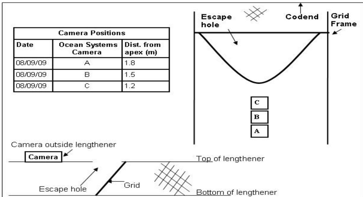
**Figure 4:** Camera placement for the three tows undertaken during initial sea trials, side and plan views.
