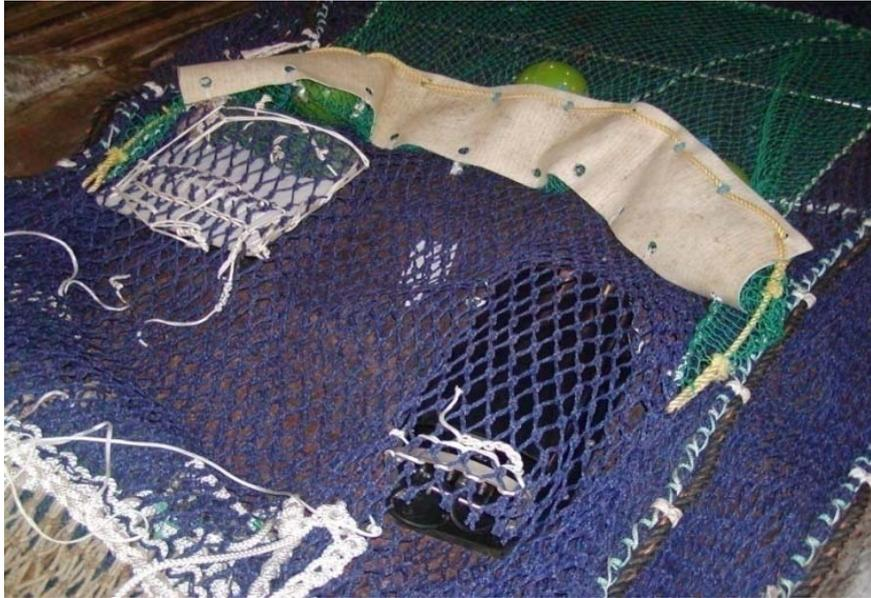
**Figure 2:** Both cameras fitted inside the SED lengthener, *FV Taimania*, April 2009
