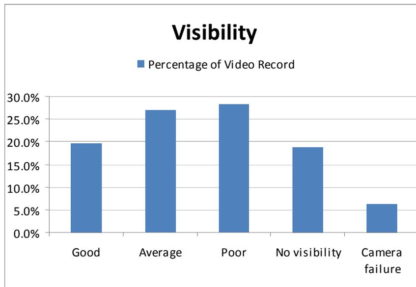
**Figure 11:** Visibility ratings as a percentage of the total 42 hours of video record of SED operation during second sea trial, April, 2009
