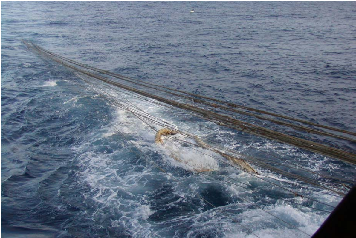
Figure 12: Head line, kite and large rope meshes, hauling onboard, FV Aleksandr Buryachenko 2008
