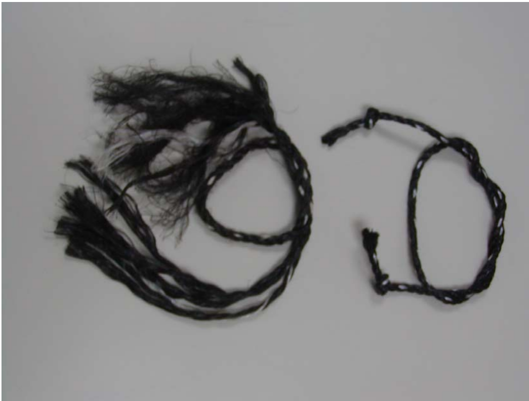
Figure 6: Mussel rope showing how it frays after use, bind on right is unused. This fraying was implicated in a failed release that ended in a wasted tow by the vessel, FV Taimania 2008
