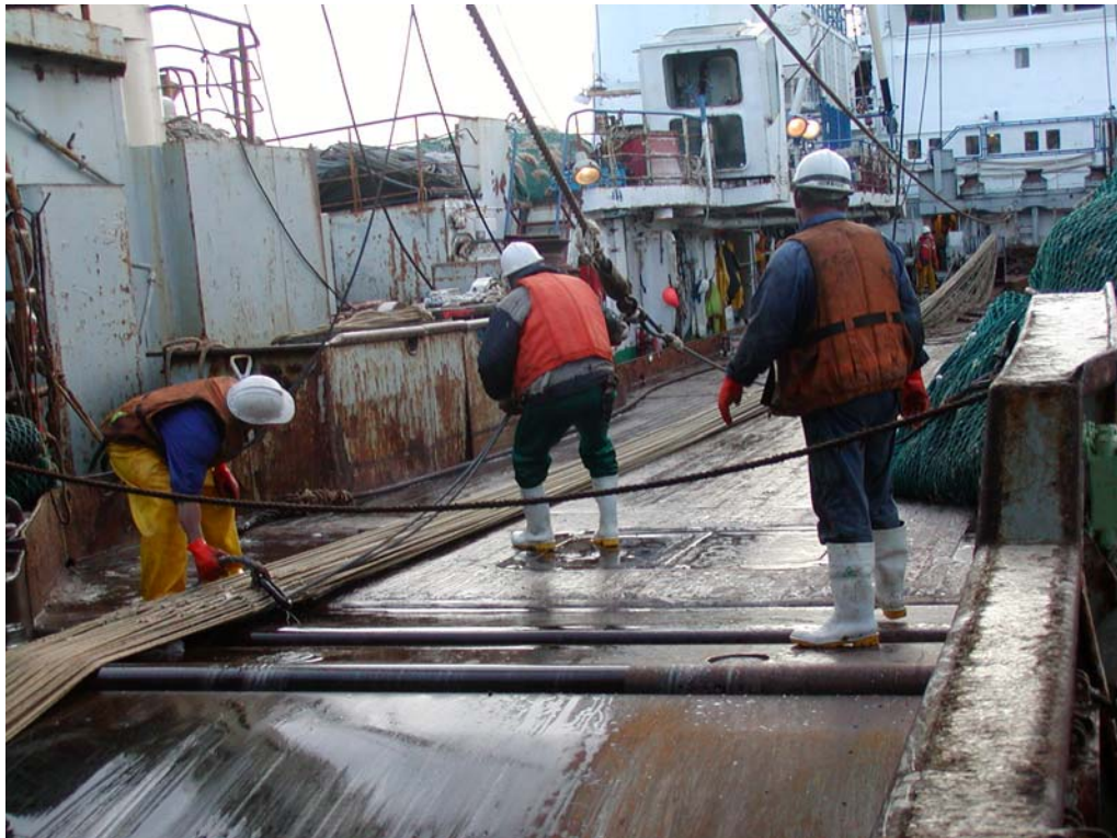
Figure 11: Crew strop and pull/winch the net in sections, fleeting it on the deck, FV Aleksandr Buryachenko 2008.
