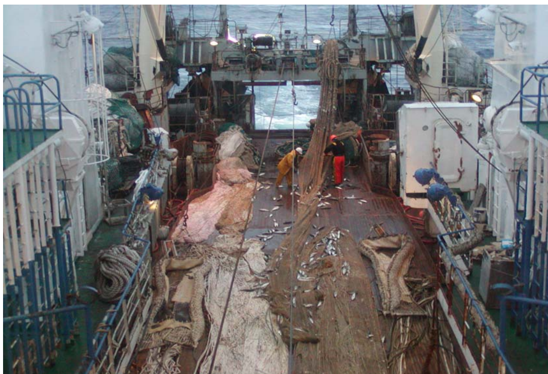
Figure 7: Trawl deck, with two midwater trawls; starboard side ready to shoot, the port net is being cleaned of stickers, FV Aleksandr Buryachenko 2008
