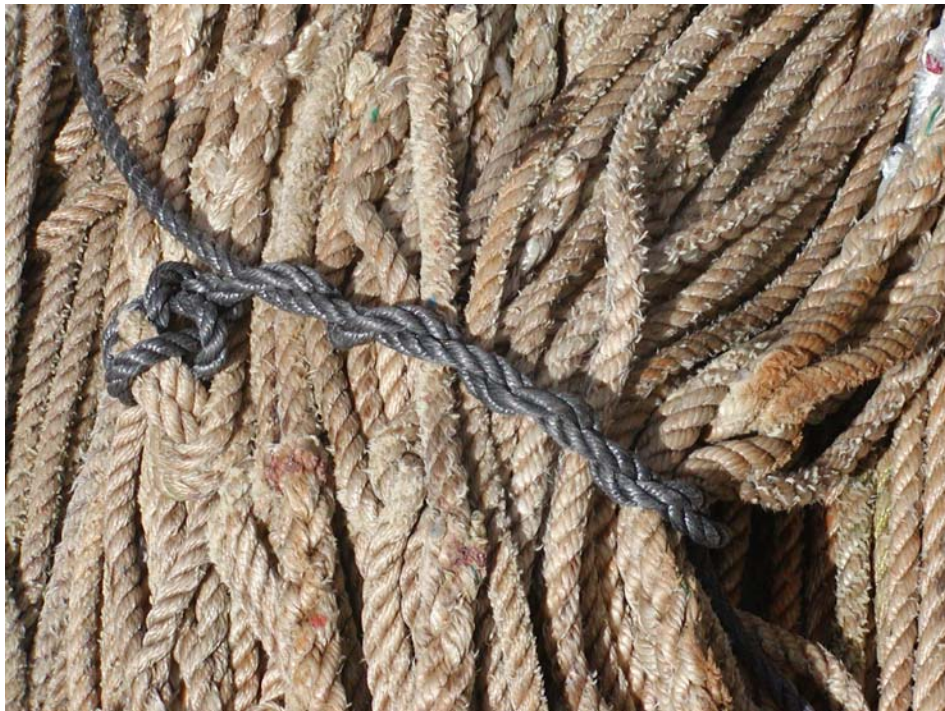
Figure 13: Binding of 10 mm PPE rope with 4 twists placed on the rope meshes, FV Aleksandr Buryachenko 2008
