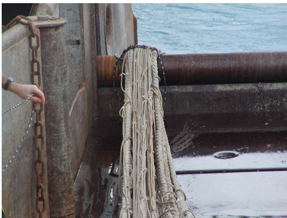
Figure 1: Midwater trawl net being shot away with synthetic rope bind visible around net as it passes over the wave gate roller, FV Taimania , 2008
