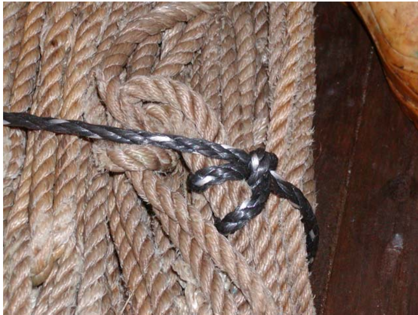
Figure 8: Mussel rope (net bind) tied to the rope mesh so it will not fall off, FV Aleksandr Buryachenko 2008
