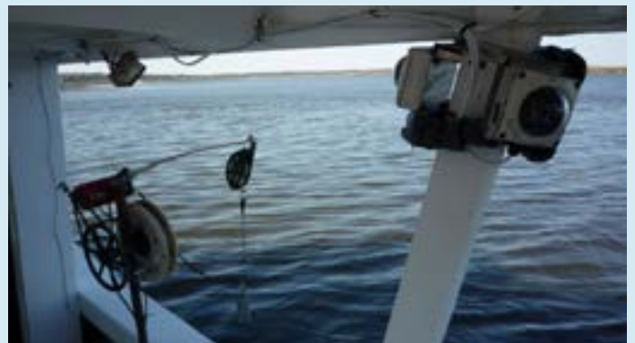
Cameras fitted on a commercial fishing vessel in the USA. Photo: https://www.st.nmfs.noaa.gov/advanced-technology/electronic-monitoring/index
