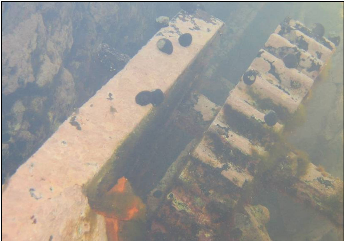
Appendix 10: Underwater image of part of the crane winch for the tramway and landing (K Upperton 2010).
