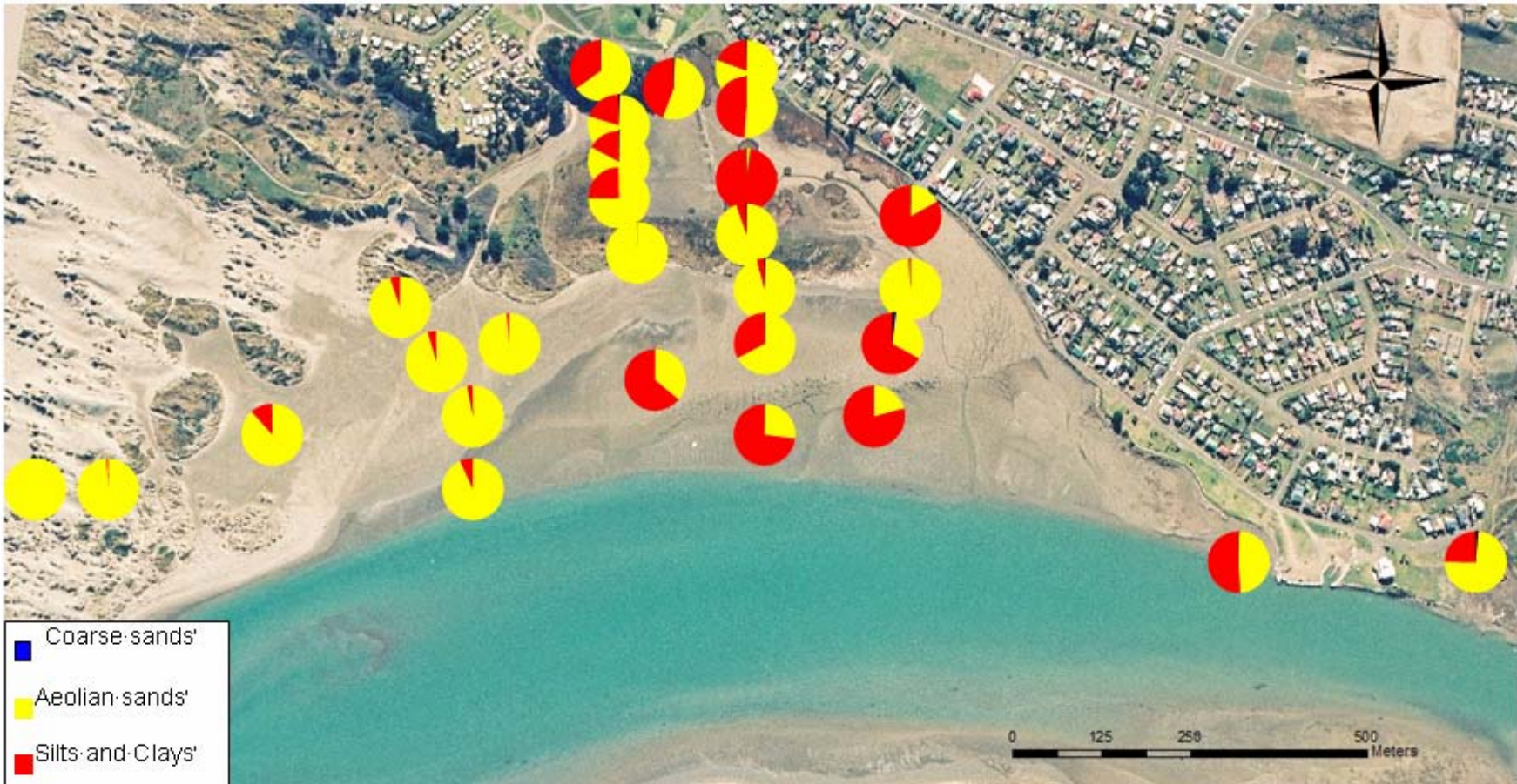
Figure 26. Map of grain size distribution along the northern bank of the Manawatu estuary. Grain size is determined in percent by weight and grouped as: coarse sand (-2 to 1.5 \phi ), dune sands (2 to 4 \phi ), and muds (<4 \phi )
