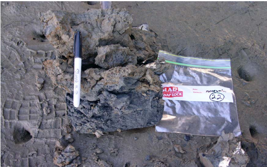
Figure 9. Sediment sampling at Site 22. Note clear boundary between the upper layer of sediment (composed of muds) and the lower sediment (composed of sands).
