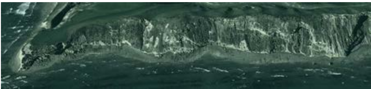
Figure 5-4: Sector 8 - Imagery from 2009 (above) and 2012 (bottom) - shallow landsliding between Jack's Camp and Black Reef due to the 2011 rainfall event
