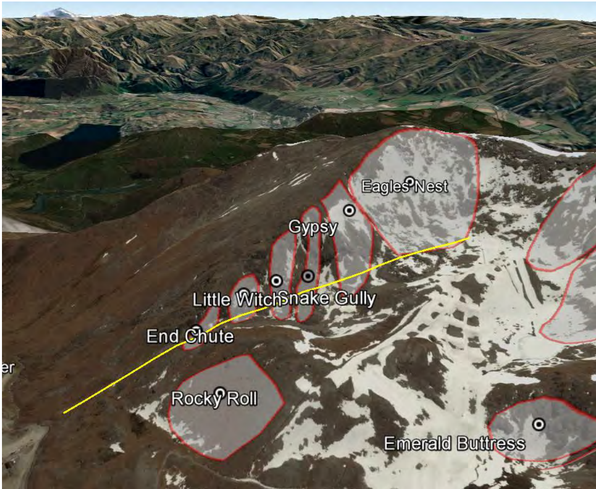
Figure 7-1: mapped avalanche paths and the lift route
