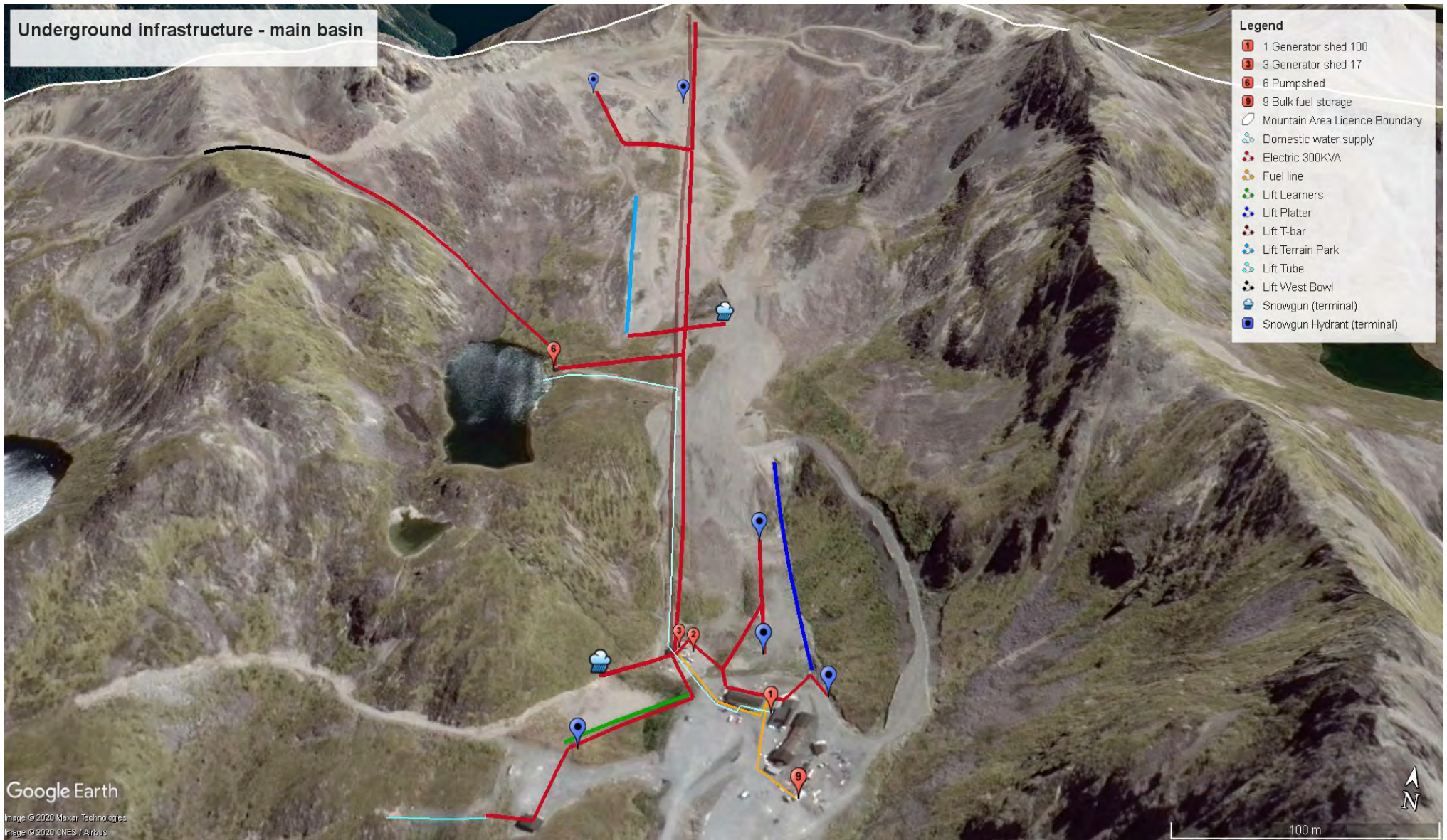
Figure 64: Underground infrastructure - main basin
