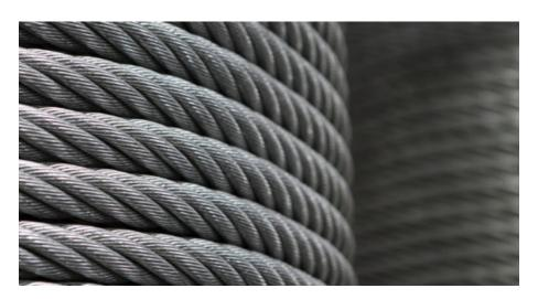
This is a photo of what 99% of zipline operators in NZ are currently using. It is cheaper but the sound is 50% greater and the lifetime is 1/8th of German-made Pfieiffer cable.
