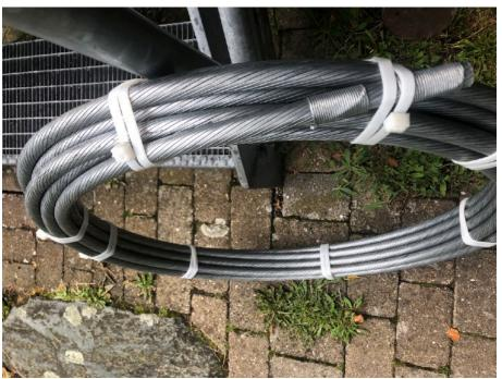
This is the style wire that we have chosen. You can see the difference in the texture. The smooth swaged surface means that not only is it more durable but also reduces the sound by 66% in comparison to a standard zipline cable.
