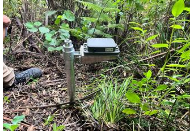
Satellite uplink from tiltmeter
