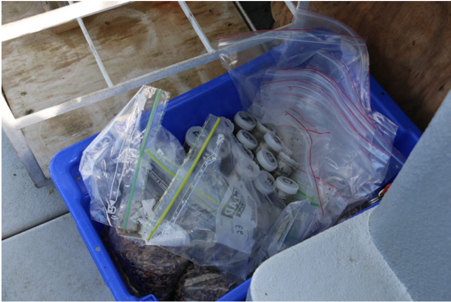
Caption: A small sediment sample was taken from each grab and the rest of each sample was put into a large snaplock bag for processing later.
