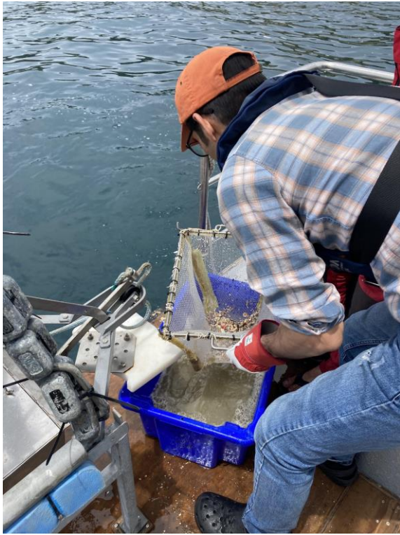
Caption: The sample then had to be sieved through a 4 mm mesh, only leaving sediment and creatures of a certain size range.
