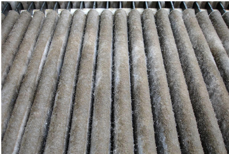
Figure 7. An AdvanTex® AX100 Filter textile after several years of operation
