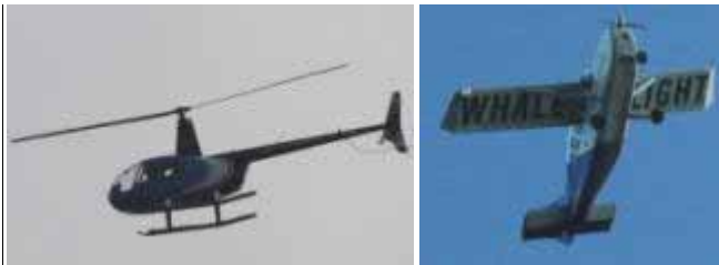
Figure 3.1. Aircraft monitored in this study included helicopters and fixed wing aeroplanes. Helicopters (left) were fitted with GPS data loggers to track their movements. Fixed wing planes (right) were either fitted with GPS data loggers (Kaikoura Aeroclub) or used their own GPS logging system which could be downloaded by researchers (Wings Over Whales). Onboard observers also collected data on some fixed wing flights.
