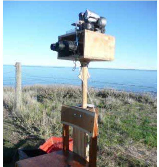
Figure 2.4. Video system. Digital video binocular system is used to monitor and track whales and vessels.
